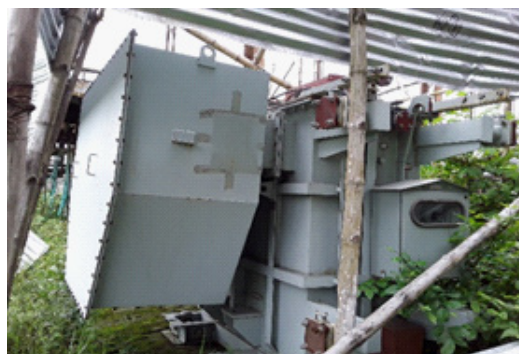
Figure 3.3: Coreless furnace lying in open field
