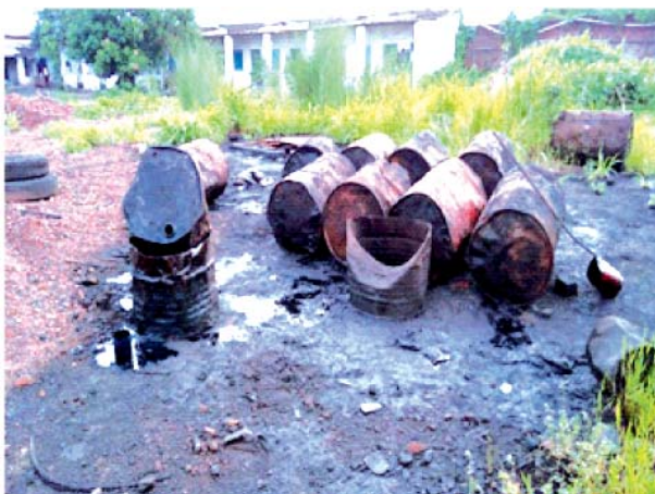
Fig 4.1 : Spillage of Oil and Grease within the premises of M/s. K. B. Sponge Iron Limited
